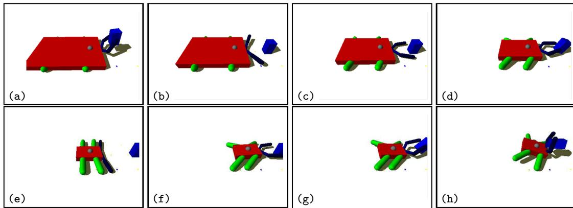
Figure 1: Results from a typical trial selecting for locomotion and object manipulation. At the outset of the trial the robot learns to grasp and lift the object (a). When the object is moved further away, the robot evolves longer legs in order to lean forward and manipulate the object (b-d). When the object is placed beyond its reach (e), it evolves to locomote to the object and then lift it (f-h).
