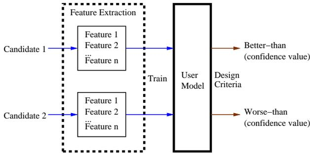
**Figure 2: The basic structure of a Comparator user model. Features are extracted from two candidate designs and are fed into the Comparator, which then uses these features to predict which one is better.**
