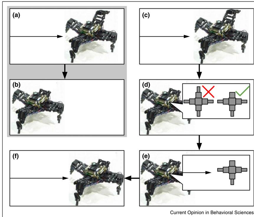
Robot prospection. A robot incapable of prospection (a) is unable to move once it suffers physical damage, such as the loss of part of a leg (b). Another robot that can move and can predict (c), once damaged, mentally simulates its situation and deduces that it has been damaged (d). It then mentally rehearses a motor program that will enable it to regain the ability to move despite its injury (e). Finally, it executes that motor program and thus autonomously recovers from the injury (f).
