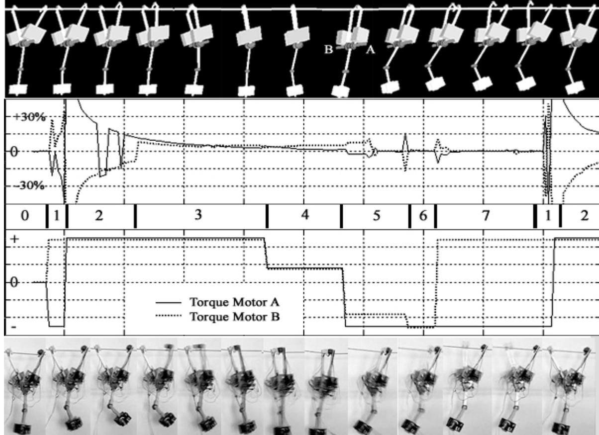
**Figure 4. Virtual locomotion cycle (top); qualitative torque analysis and phase definition (centre); real world locomotion cycle (bottom). Agents are moving to the left, the time axes is read to the right. Positive torque-axis oriented towards the reader with the origin in the middle section of the upper body. Motor A pointing towards the reader.**
