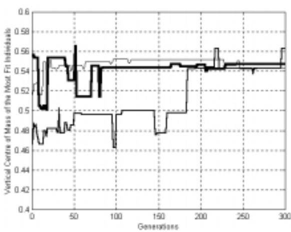
Figure 9: Changes in vertical position of biped Center of Mass: The thin line tracks the changes of the vertical CoM for the most fit biped in the microscopic case. The middle line tracks the CoM of the best biped in the mid-range case and the thick line is that of the best biped in the macroscopic case.
