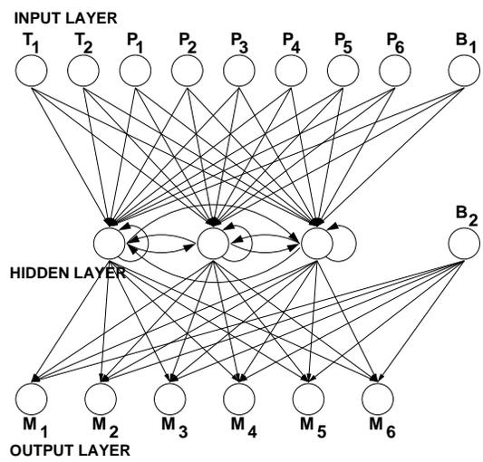
Figure 2: gives a pictorial representation of the neural network used to control both types of agents. T1 and T2 correspond to the two touch sensors, P1 through P6 indicate the six proprioceptive sensors, and M1 through M6 indicate the six torsional motors of the biped. B1 and B2 indicate the two bias neurons included in the network.
